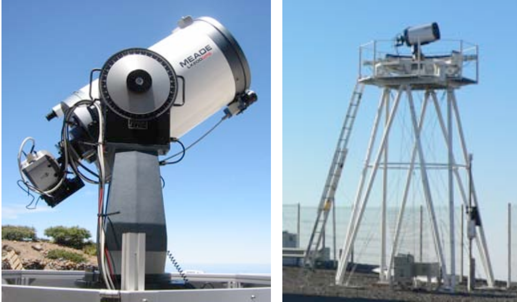
Fig. 1: Left: Durham/ESO prototype SLODAR System. Right: The SLODAR instrument transferred to an Astelco NTM100 mount and tower/enclosure (E-ELT site testing equipment) at Cerro Paranal for a test of fully robotic operation (2007).
