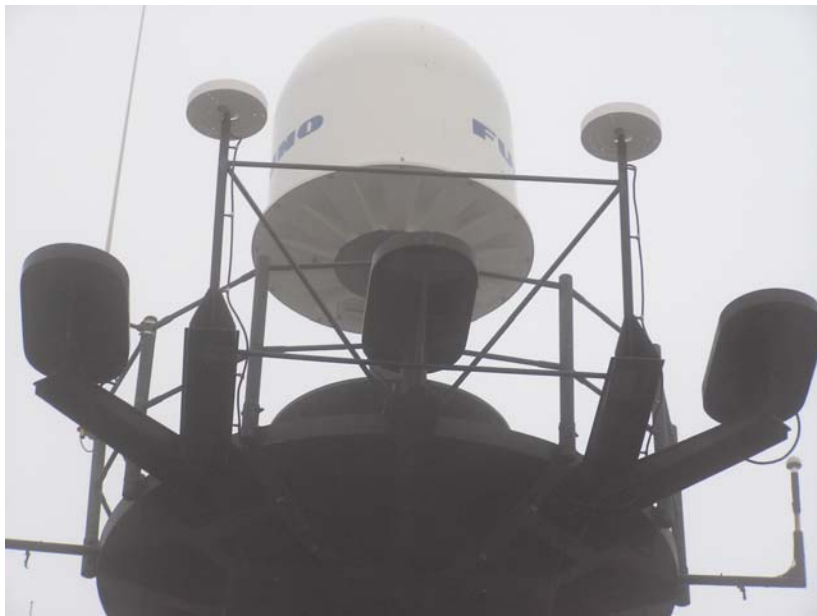
Figure 7- POS/MV antennas mounted on the main mast (view from bow).
