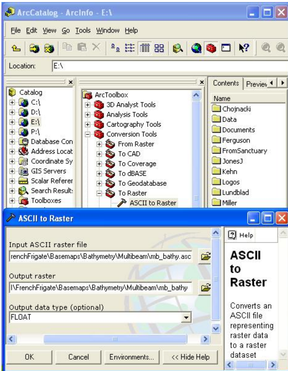
Figure 5: ASCII files are converted to Arc Raster grids for use in GIS analysis and maps.
