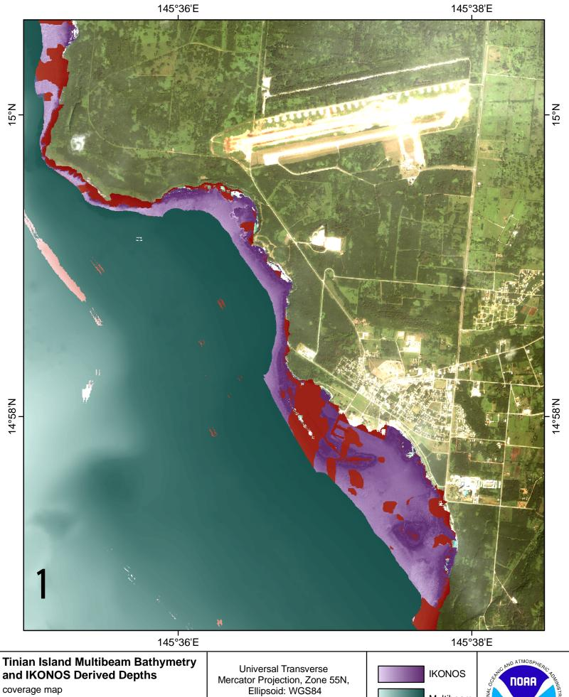
Data include NOAA Ship Hi'ialakai and R/V AHI multibeam bathymetry, IKONOS image by Space Imaging. Satellite image form USGS DOQQ. LIDAR from SHOALS-400 algorithm NOT FOR NAVIGATION
