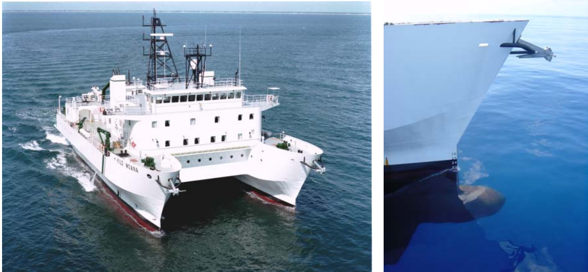
Fig. 12. R/V Kilo Moana on mission trials in the Atlantic (left, KiMo website) and close-up of the port hull bow showing submarine-like shape, stabilizing canard (fin) and small air-water interface (from P. Johnson).
