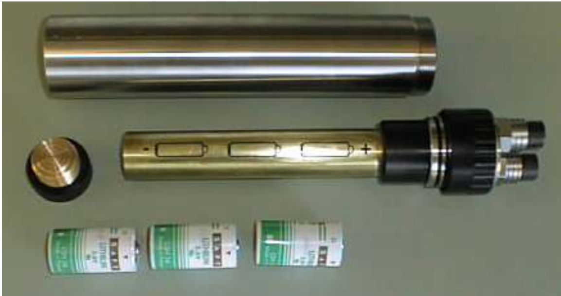
Figure 4.3.2.1 The Battery pack
