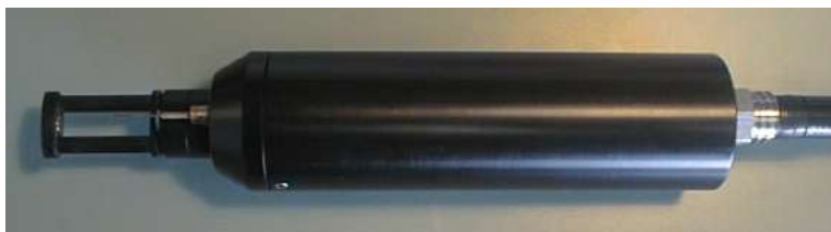
Figure 1.1: Micro SVT with optional 85ms temperature sensor
