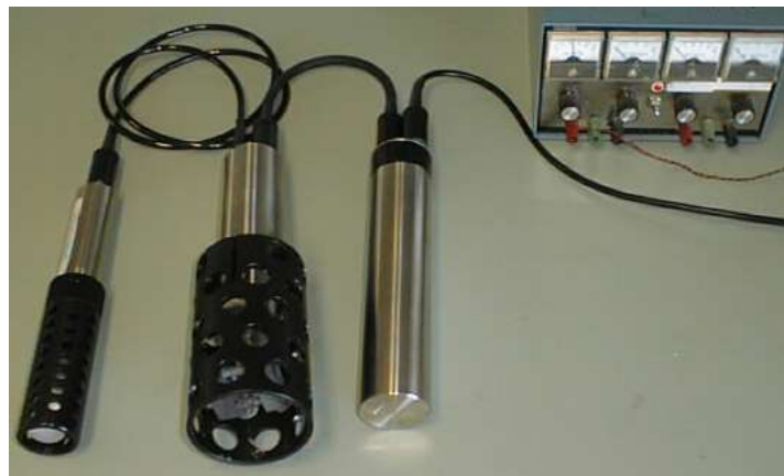
Figure 4.3.2 Micro instrument with battery pack and external sensor connected to an external power supply
