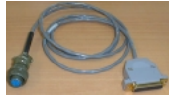
NMEA Interface test cable (NMEA Interface Box to NMEA navigation device simulation computer)
