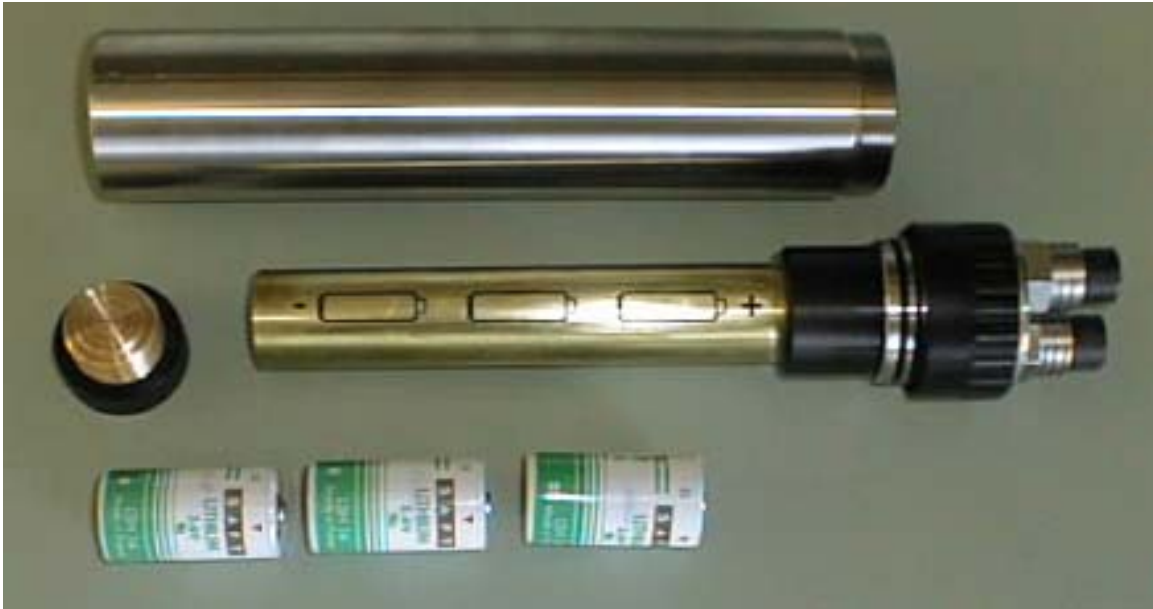
Figure 4.3.2.1 The Battery pack
