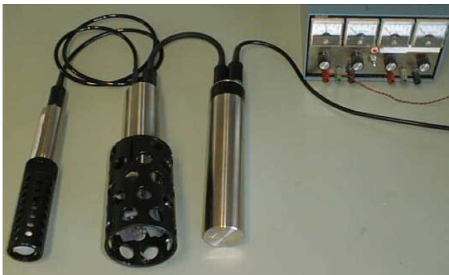
Figure 4.3.B The Micro CTD with battery pack and external sensor connected to an external power supply.
