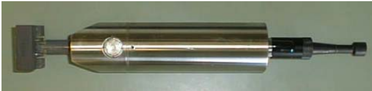
Figure 1.1: Micro CTD Sensor with Optional Stainless Steel Pressure Case
