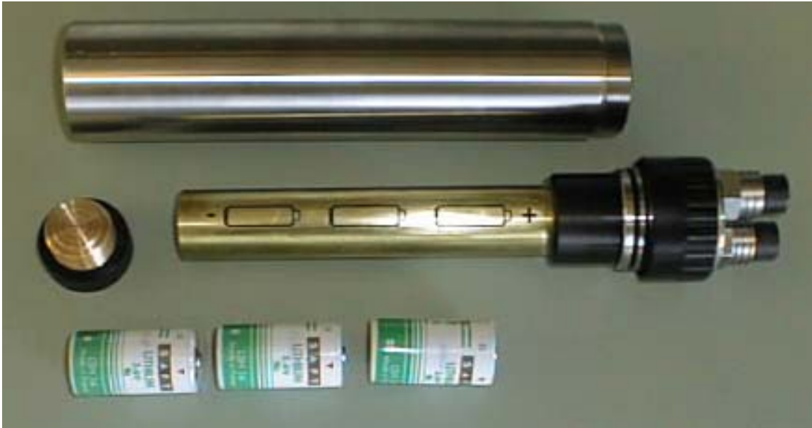
Figure 4.3.1 The Battery pack
