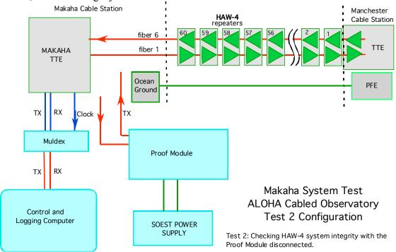
ALOHA Cabled Observatory Proof Module System Test Page 2 of 11 3) Connect fibers 1 and 6 (primary fiber pair) to the Proof Module and loop back these fibers at Manchester so that data and commands travel from Makaha to Manchester and back, establishing an 8,000 km data path length.
