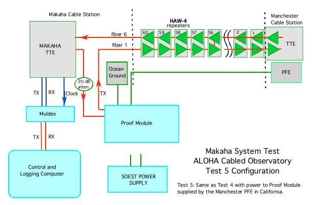
6) Cycle the cable power at Manchester and evaluate how the Proof Module reacts to the power cycle.
