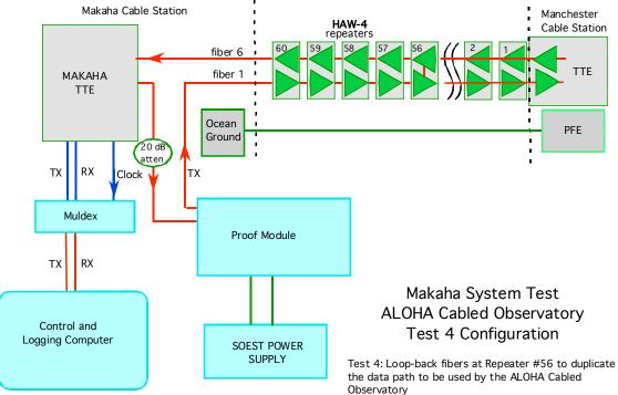
ALOHA Cabled Observatory Proof Module System Test Page 3 of 11 5) Use the cable power supplied from Manchester to power the Proof Module and evaluate.
