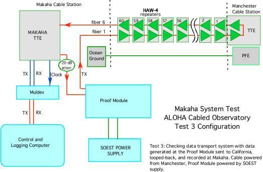
4) Loop-back fibers 1 and 6 at repeater 56, north of Station ALOHA, to simulate the length of the projected cable path.
