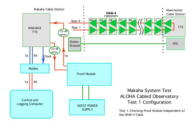
2) Power-up the HAW-4 cable from Manchester and evaluate the HAW-4 system, repeaters, and data integrity.
