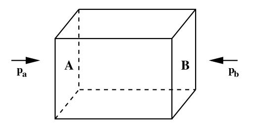
If  $p_A = p_B$ , where  $p_n$  is the pressure exerted on a given side of the fluid element, then there is no net force acting on the fluid element.
