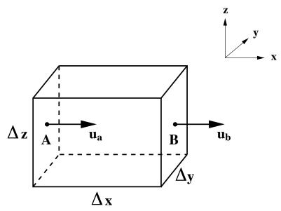
The mass flux (flow per unit time) out of box through side B is
