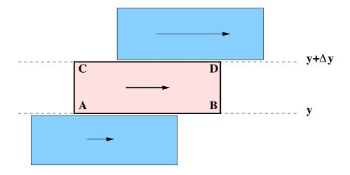
The faster fluid above **AB** will drag forward the slower moving fluid below, and visa versa.
