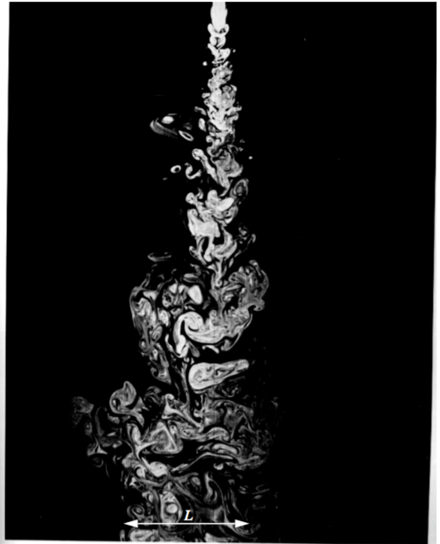
166. Turbulent water jet. Laser-induced fluorescence shows the concentration of jet fluid in the plane of symmetry of an axisymmetric jet of water directed downward into water. The Reynolds number is approximately 2300.
