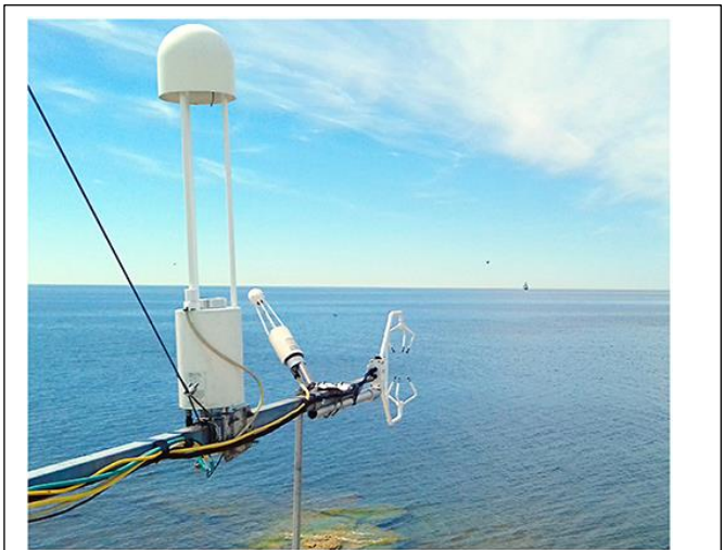
Figure 4. Eddy covariance system for methane in Baltic sea. Photo from Gutiérrez-Loza et al., 2019.
