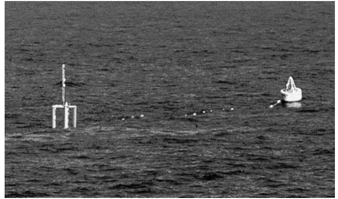
Figure 1. Photograph of the ASIS (left) and tether buoys deployed during FETCH. For scale, the mast on ASIS has a height of 4 m.
