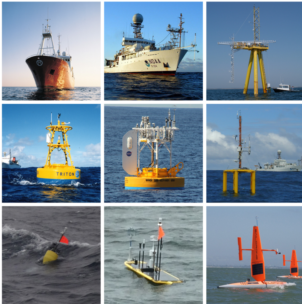
FIGURE 3 | Examples of different types of air-sea flux in situ platforms. Clockwise from upper left: Norwegian weather ship Polarfront (image courtesy of Norwegian Meteorological Institute) (Yelland et al., 2009); NOAA ship Ron Brown (from www.noaa.gov ); WHOI Air-Sea Interaction Tower (image courtesy Jayne Doucette Woods Hole Oceanographic Institution); RSMAS “ASIS” spar buoy (Graber et al., 2000); Saildrone, Inc., “Saildrone” ASV (image courtesy of Saildrone, Inc.; www.saildrone.com ), Liquid Robotics “Wave Glider” ASV (from www.liquid-robotics.com with modifications by UW/APL), UW/APL “SWIFT” drifter (Thomson, 2012); JAMSTEC TRITON buoy (from JAMSTEC, www.jamstec.go.jp ); and, in the center, the WHOI SPURS buoy (Farrar et al., 2015).
