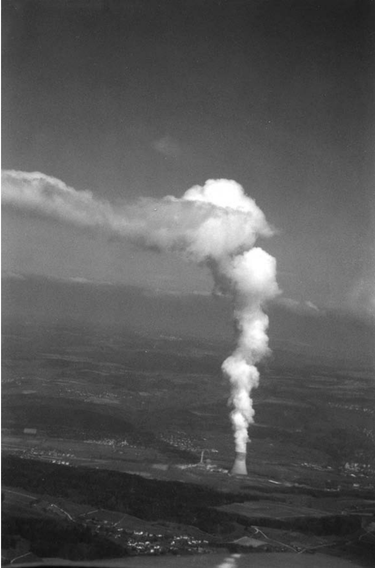
Figure 1.8. A plume rising over the nuclear power plant at Gosgen, Switzerland, in the Swiss Foothills. The plume rises, eddies at its edge entraining surrounding air, until it meets and spreads on an inversion (a stably stratified layer). (Photograph kindly provided by Paul E. Oswald.)
