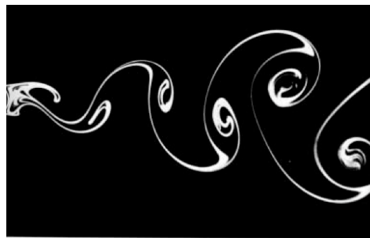
94. Kármán vortex street behind a circular cylinder at Re=140 . Water is flowing at 1.8 \text{ cm/s} past a cylinder of diameter 1 cm. Integrated smalltime are shown by electrolytic precipitation of a white colloidal smoke, illuminated by a sheet of light. The vortex street is seen to grow in width downstream for some diameters. Photograph by Saku ōno/Tanaka van Dyke, p. 56
