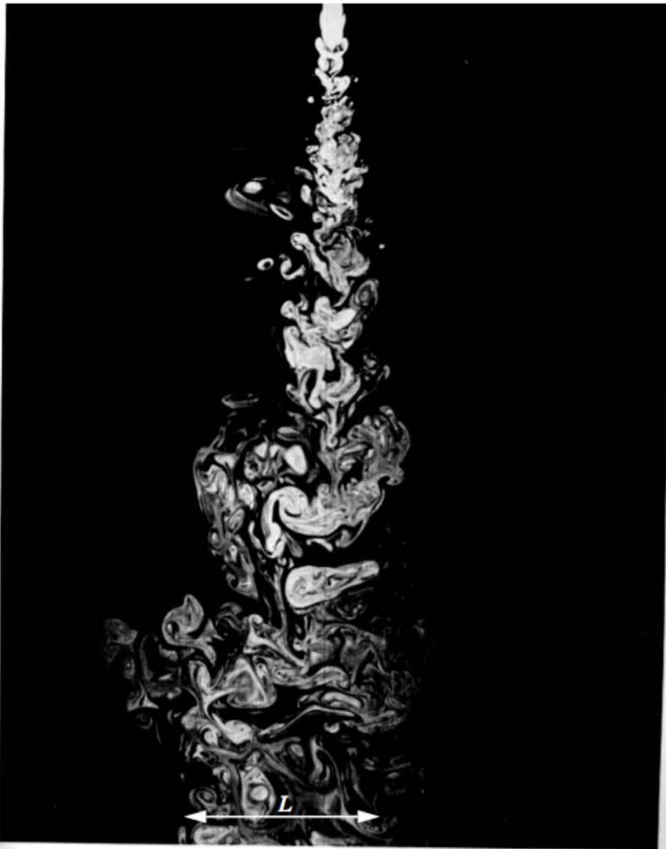
166. Turbulent water jet. Laser-induced fluorescence shows the concentration of jet fluid in the plane of symmetry of an axisymmetric jet of water directed downward into water. The Reynolds number is approximately 2300.
