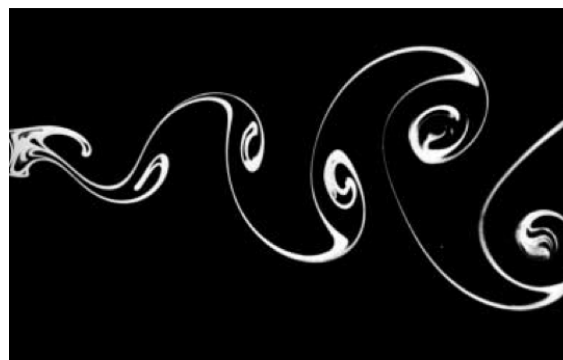
94. Kármán vortex street behind a circular cylinder at Re=140 . Water is flowing at 1.8 cm/s past a cylinder of diameter 1 cm. Integrated streaklines are shown by electro-lytic precipitation of a white colloidal smoke, illuminated by a sheet of light. The vortex street is seen to grow in width downstream for some diameters. Photograph by Saku Inohé Taniada
