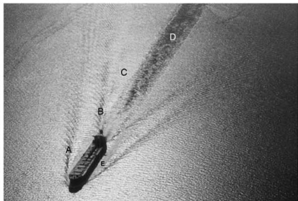
Fig. 7.13 Photograph of a ship and its wake in Chesapeake Bay near Annapolis, MD, showing classic Kelvin and turbulent wakes. Wake components: a bow wave, b stern wave, c transverse wave, d turbulent wake, and e turbulent region adjacent to ship. (After Pichel et al. (2004). (Copyright © 2004 NOAA)
