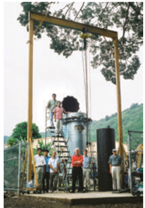
Flash Carbonization™ producing charcoal from biowaste
