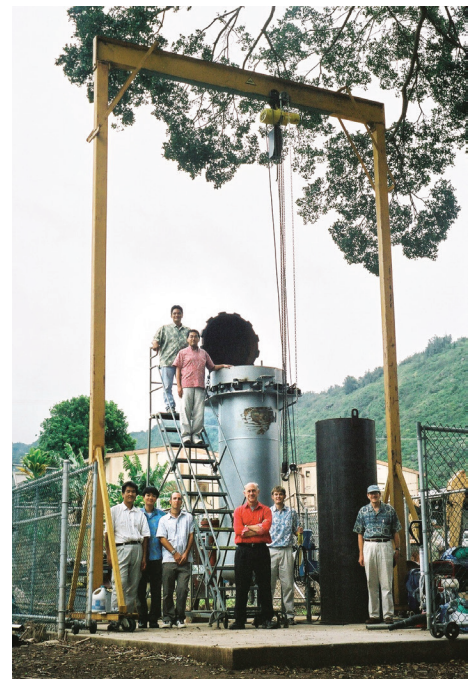
Flash Carbonization™ producing charcoal from biowaste
