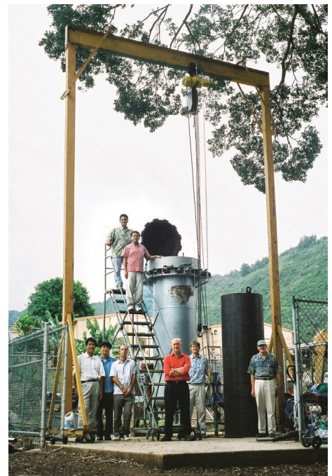
Flash Carbonization™ producing charcoal from biowaste
