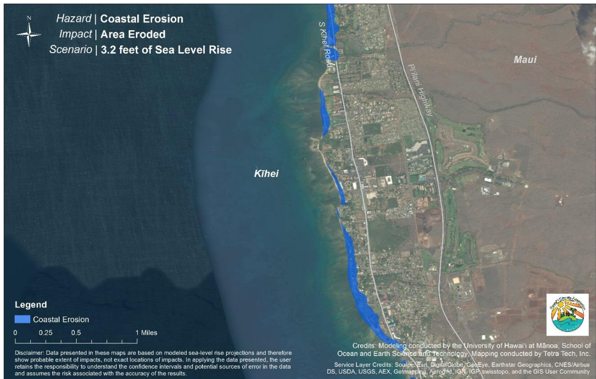
Figure 28. Example maps showing the results of coastal erosion modeling with 1.1 feet (top) and 3.2 feet (bottom) of sea level rise for Kīhei, Maui
