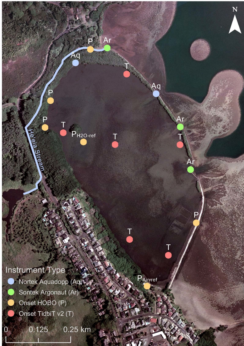
Figure 1.10. Instrument deployment locations: Nortek Aquadopp (Aq), Sontek Argonaut (Ar), Onset HOBO water level logger (P), Onset TidBit v2 temperature logger (T).
