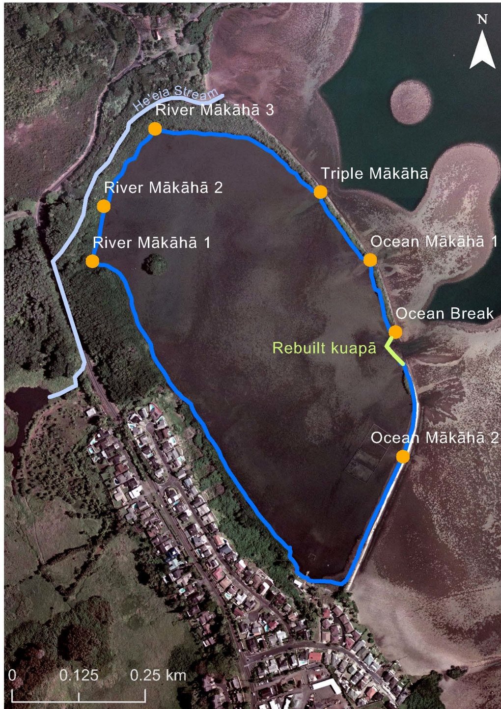
Figure 1.4. He'eia Fishpond perimeter and mākāhā (sluice gates). Three freshwater mākāhā: River Mākāhā 1 (RM1), River Mākāhā 2 (RM2), and River Mākāhā 3 (RM3). Three saltwater mākāhā: Triple Mākāhā (TM), Ocean Mākāhā 1 (OM1), and Ocean Mākāhā 2 (OM2). Rebuilt kuapā (fishpond wall): Ocean Break (OB).
