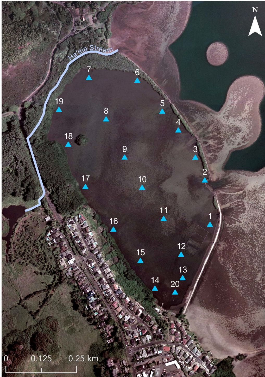
Figure 1.6. He'eia Fishpond permanent stake (1-20) locations. The monthly sampling plan collected water samples at stakes 1, 3, 6, 7, 8, 9, 13, 15, 16, and 18.
