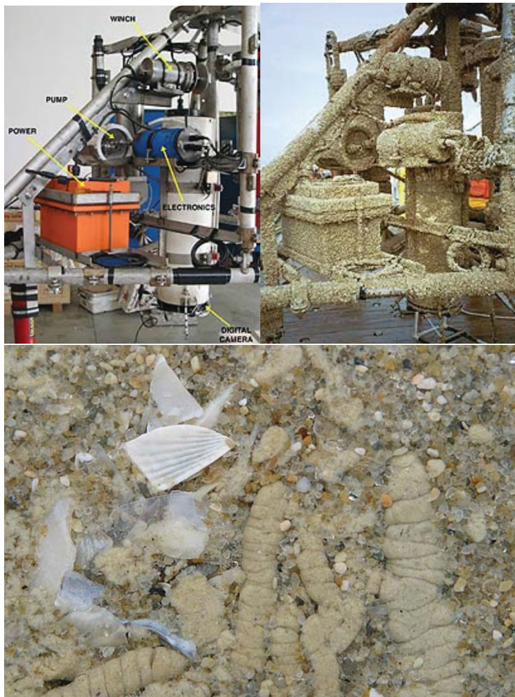
Figure II.F.1. USGS autonomous "Poking Eyeball" seabed camera system. To periodically sample the bottom, a winch automatically lowers a digital camera to the sea bed until sediment grains are pushed right up to the window on the camera housing. (upper left) Just before deployment, (upper right) after 101 days on the seafloor, (lower) example image (7 mm across) from a 9-m site in the Adriatic Sea. The extreme biofouling emphasizes the potential environmental disturbance associated with any seabed instrumentation. From Chezar and Rubin (2003) and Sherwood (2003).
