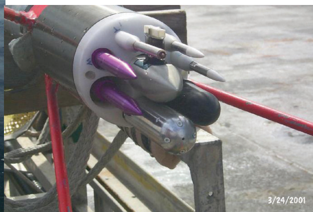
Figure II.F.2. Freely-falling turbulence profiler, Chameleon (left), developed and operated by the Ocean Mixing Group at Oregon State University to rapidly profile the coastal ocean. Chameleon has sensors (below) to measure pressure, temperature, conductivity and velocity fluctuations on the small scales of ocean turbulence. She also has sensors to measure optical backscatter and chlorophyll fluorescence. She is routinely deployed to crash into the ocean floor (using the sensor protection ring shown), yielding profiles of all quantities to within 2 cm of the bottom. Figures courtesy of Jim Moum.
