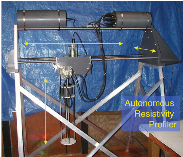
Figure II.F.8. An autonomous resistivity profiler capable of relocating the position of the probes to facilitate repeated measurements in sediments without extensive disturbance.
