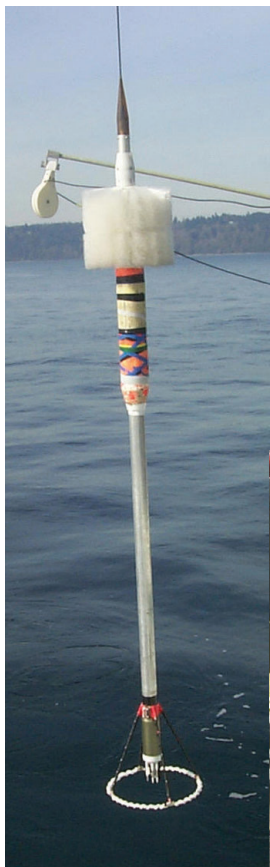
Figure II.F.2. Freely-falling turbulence profiler, Chameleon (left), developed and operated by the Ocean Mixing Group at Oregon State University to rapidly profile the coastal ocean. Chameleon has sensors (below) to measure pressure, temperature, conductivity and velocity fluctuations on the small scales of ocean turbulence. She also has sensors to measure optical backscatter and chlorophyll fluorescence. She is routinely deployed to crash into the ocean floor (using the sensor protection ring shown), yielding profiles of all quantities to within 2 cm of the bottom. Figures courtesy of Jim Moum.
