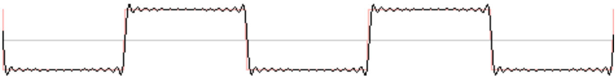
Figure II.5. Square wave function representation as a sum of sinusoids.
