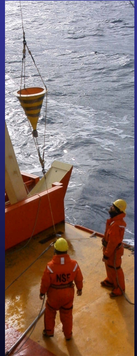
SEDIMENT TRAP RECOVERY
